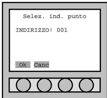
The image shows a rectangular menu box with a double border. Inside, the text 'Selez. ind. punto' is at the top. Below it, 'INDIRIZZO: 001' is displayed. At the bottom left of the inner box are two buttons labeled 'Ok' and 'Canc'. Below the main menu box is a horizontal row of four circular indicators, each with a vertical line through its center, representing a loop selection.
