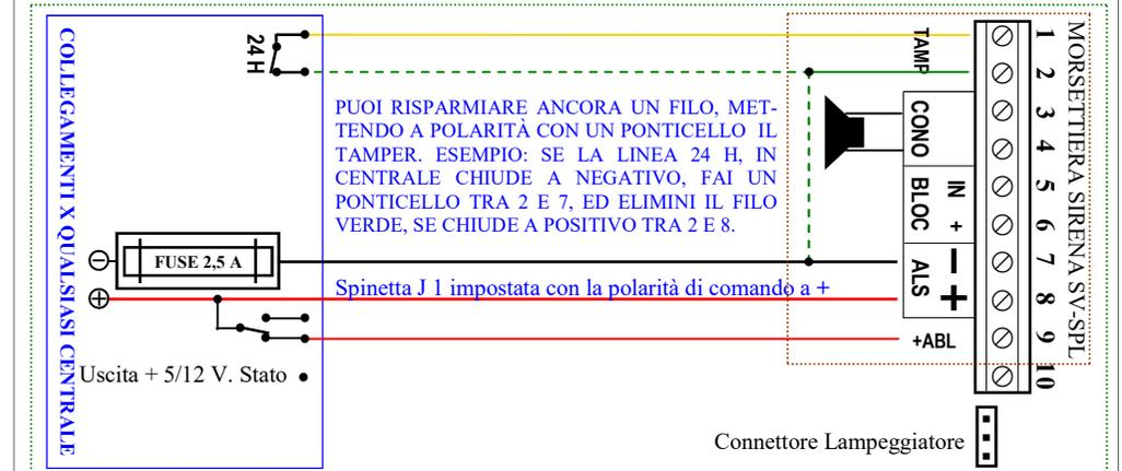
PUOI RISPARMIARE ANCORA UN FILO, METTENDO A POLARITÀ CON UN PONTICELLO IL TAMPER. ESEMPIO: SE LA LINEA 24 H, IN CENTRALE CHIUDE A NEGATIVO, FAI UN PONTICELLO TRA 2 E 7, ED ELIMINI IL FILO VERDE, SE CHIUDE A POSITIVO TRA 2 E 8.
